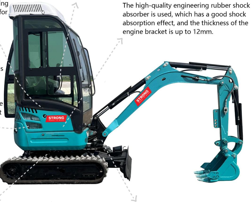
The high-quality engineering rubber shock absorber is used, which has a good shock absorption effect, and the thickness of the engine bracket is up to 12mm.
