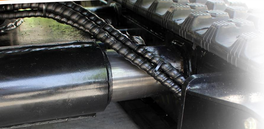
The bottom plate is retractable, widening the bottom plate can make walking more stable, shortening the bottom plate, can enter the narrow road, can be expanded and retracted arbitrarily according to your own requirements, and the work is not
